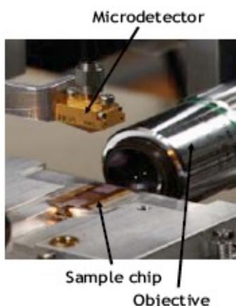
Fig.1. Sample chip in Vibratess' Spectrometer, Vibr-2, for general laboratory applications. [1]
